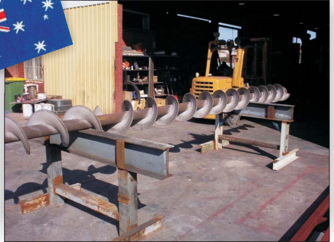
Conveyor after grit blasting
