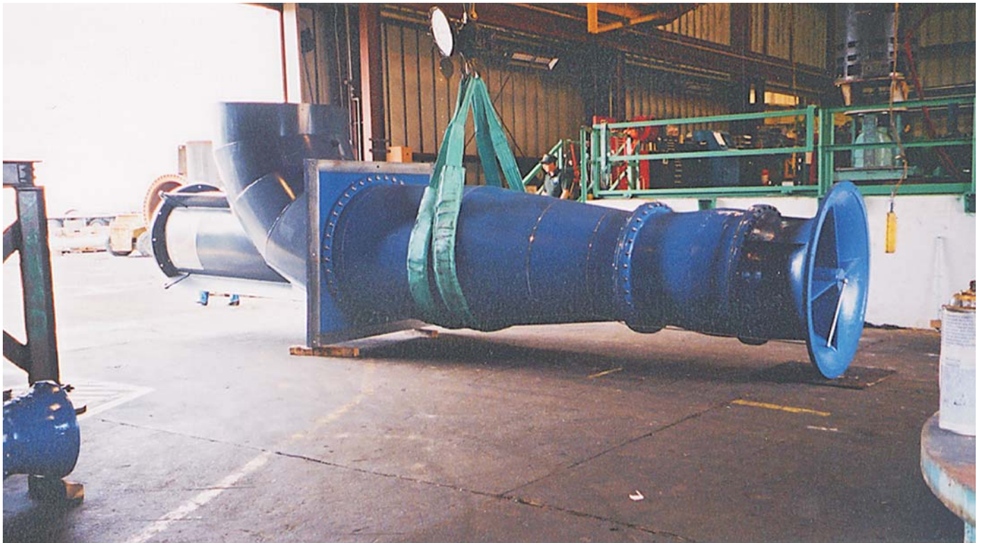
Completed Pump System: includes over 50 ENECON coated parts.
