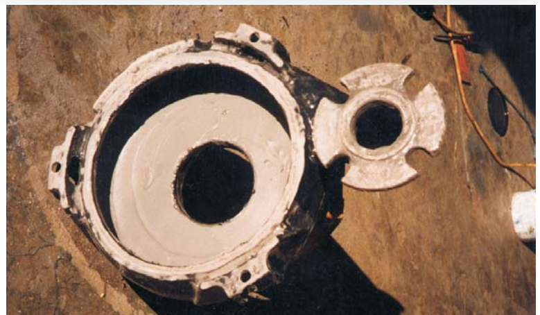
CeramAlloy CP+ was used to rebuild all damaged surfaces.
